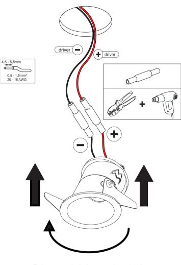
Twist counterclockwise to put through hole then twist clockwise to fixate
