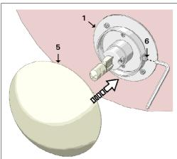
Screw diffuser (5) to the lamp body (1) and fix it by tightening dowel (6).
