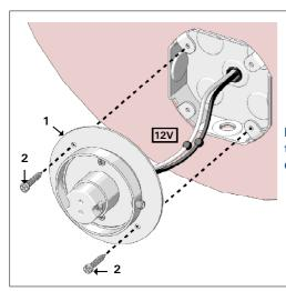
Make the electrical connections by connecting the white cable coming from the fixture to the white cable of the j-box and the black cable coming from the fixture to the black cable of the j-box. Fasten the lamp body (1) to the j-box by means of screws (2).
