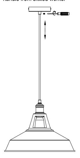
If the external flexible cable or cord of this luminaire is damaged, it shall be exclusively replaced by the manufacturer or his service agent or a similar qualified person in order to avoid a hazard.
