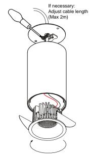
install : Twist clockwise uninstall : Twist counterclockwise
