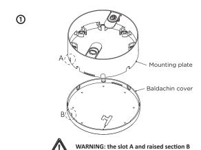
should be aligned when installation.
